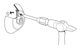
A ventilation valve can be connected at the thread connection of the suction cups  $\emptyset$  100, 150, 225 and 300. For this, the plug must be knocked from the material with a hammer and mandrel.
