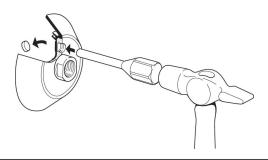
A ventilation valve can be connected at the thread connection of the suction cups  $\emptyset$  100, 150, 225 and 300. For this, the plug must be knocked from the material with a hammer and mandrel.
