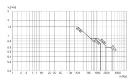
v<sub>t</sub> = Piston velocity [m/s] m = Cushionable mass [kg]
