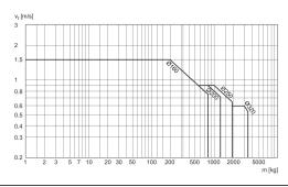
$v_t$  = Piston velocity [m/s] m = Cushionable mass [kg]
