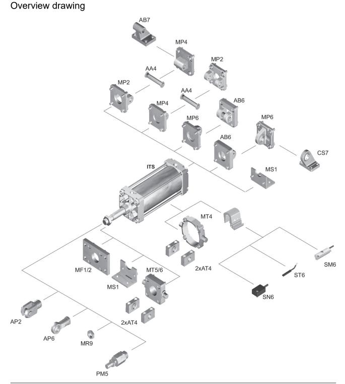
NOTE: This overview drawing is only for orientation to indicate where the various accessory parts can be fastened to the cylinder. The illustration has been simplified for this purpose. It is thus not possible to derive the dimensions from this overview.
