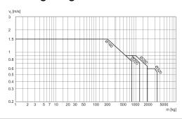
$v_t$  = Piston velocity [m/s] m = Cushionable mass [kg]
