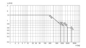
v<sub>t</sub> = Piston velocity [m/s] m = Cushionable mass [kg]
