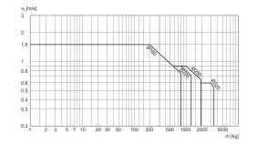
v<sub>t</sub> = Piston velocity [m/s] m = Cushionable mass [kg]
