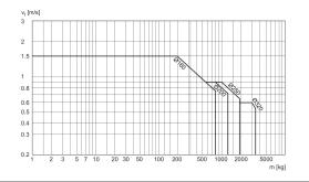
$v_t$  = Piston velocity [m/s] m = Cushionable mass [kg]
