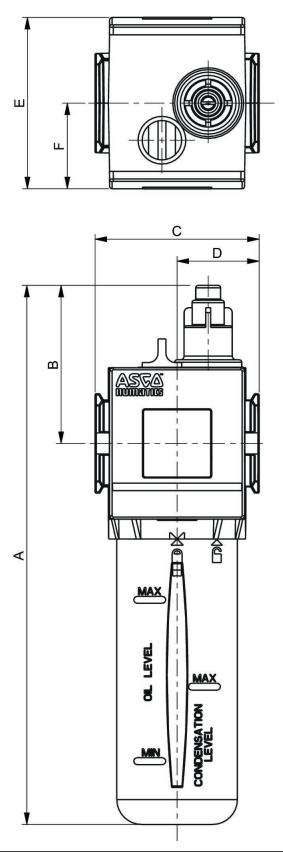
To remove the reservoir, allow a clearance of [[25] mm] from the bottom of the reservoir drain.
