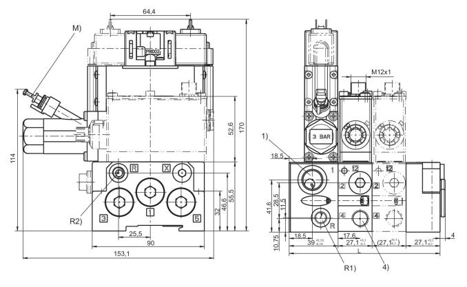
1) Operating pressure 4) Port 4 (to nozzle) R1) Test module exhaust/sealing air connection (max. [[1] bar]) R2) Pilot control exhaust M) Push-in fitting for plastic tubing Ø 6x1 of the pressure gauge
