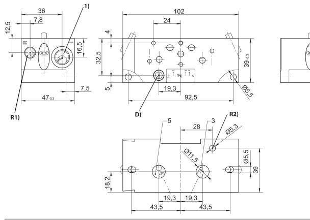
1) Operating pressure D = Throttle (cleaning pressure) R1) Test module exhaust/sealing air connection (max. [[1] bar]) R2) Pilot control exhaust
