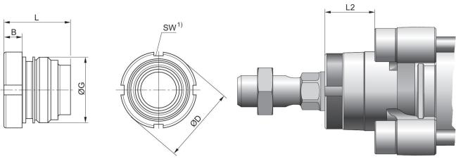
1) Can be mounted with hook wrench in accordance with DIN 1810 A
