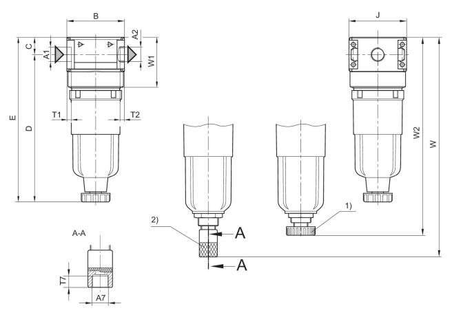
A1 = input A2 = output 1) Semi-automatic condensate drain 2) fully automatic condensate drain
