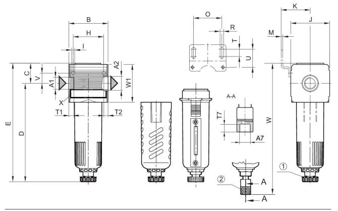
A1 = input A2 = output A7 = condensate drain 1) Semi-automatic condensate drain 2) fully automatic condensate drain
