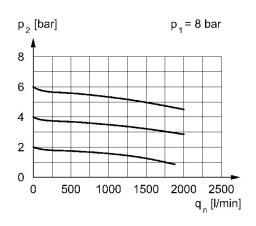
p1 = Working pressure p2 = Secondary pressure qn = Nominal flow p2 = 0.5 - 10 bar
