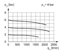
p1 = Working pressure p2 = Secondary pressure qn = Nominal flow p2 = 0.2 - 6 bar
