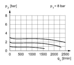
p1 = Working pressure p2 = Secondary pressure qn = Nominal flow p2 = 0,1 - 3 bar
