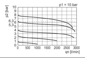
p1 = Working pressure p2 = Secondary pressure
