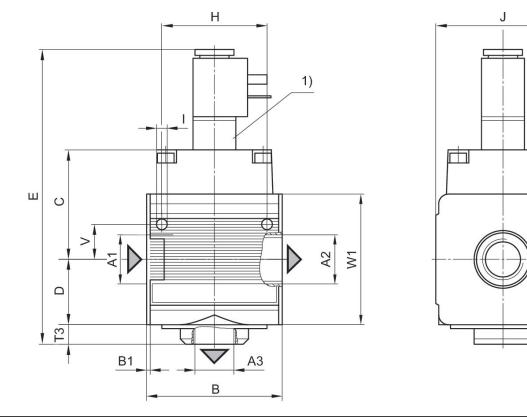
A1 = input A2 = output A3 = output 1) electrically operated
