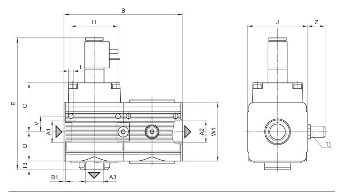
A1 = input A2 = output A3 = output 1) Adjustment screw for filling time
