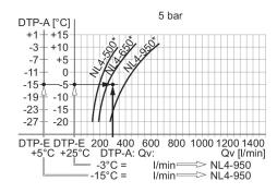
Result: membrane dryer series NL4-950 (with a Qn of 950 l/min), part no. R412007608
