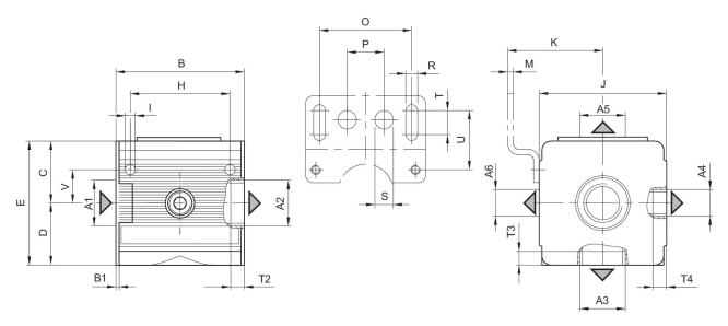
A1 = input A2 = output A3 = output A4 = output A5 = output A6 = output
