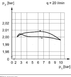
p1 = Working pressure p2 = Secondary pressure
