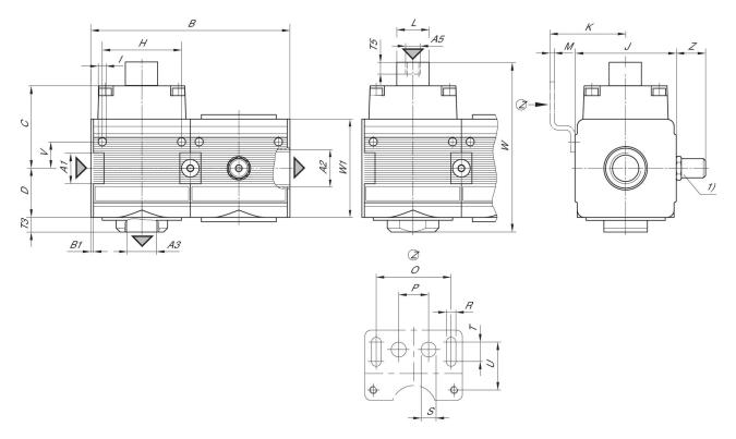
A1 = input A2 = output A3 = ventilation port A3 = ventilation port A5 = Control pressure connection 1) Adjustment screw for filling time
