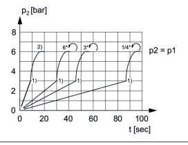
p1 = Working pressure p2 = Secondary pressure t = filling time, adjustable via adjustment screw (throttle)
