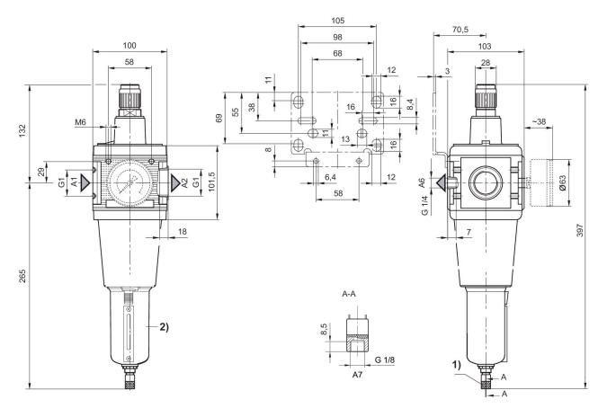
A1 = input A2 = output A6 = output A7 = condensate drain 1) Fully automatic condensate drain 2) Metal reservoir with inspection glass
