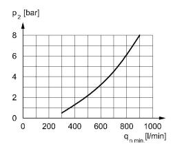
p2 = Secondary pressure qn min. = min. nominal flow
