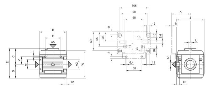
A1 = input A2 = output A5 = Control pressure connection A6 = ventilation port
