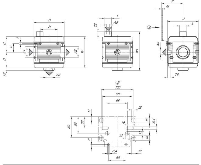
A1 = input A2 = output A3 = ventilation port A5 = Control pressure connection A6 = output
