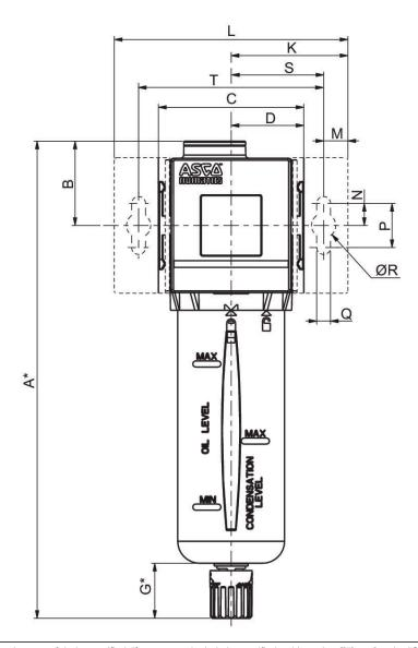
\*Variable dimension based on the type of drain specified, if an automatic drain is specified, add another [[5] mm] to the "G" dimension, which also adds 5 mm to the "A" dimension.
