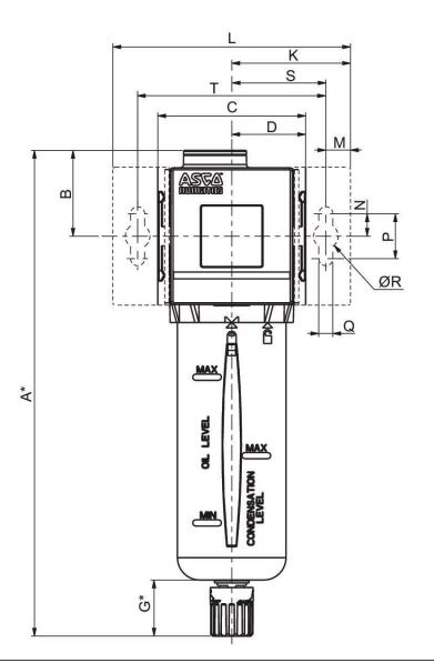
\*Variable dimension based on the type of drain specified, if an automatic drain is specified, add another [[5] mm] to the "G" dimension, which also adds 5 mm to the "A" dimension.
