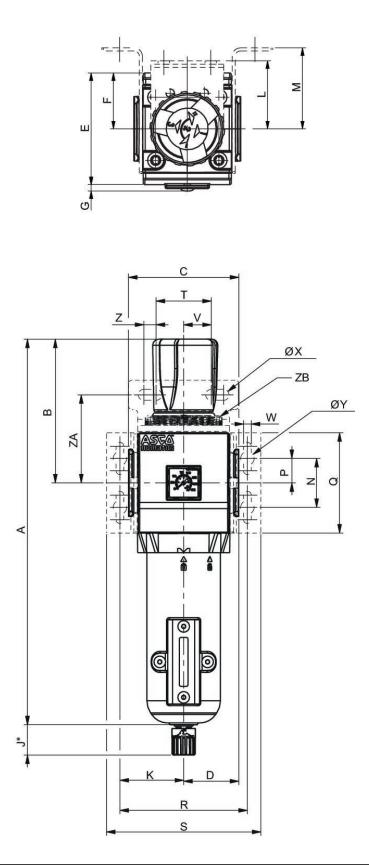
To remove the reservoir, allow a clearance of [[105] mm] from the bottom of the reservoir drain. \*Variable dimension based on the type of drain specified, if an automatic drain is specified, add another [[5] mm] to the "J" dimension.
