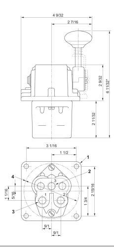
1) 9/32 diameter (4) places 2) Air supply 3) panel mounting hole Ø3 3/8 4) 1/4 - 18 NPTF \*Also available with handle 2" longer **3-position handle, detented**
