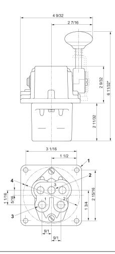
1) 9/32 diameter (4) places 2) Air supply 3) panel mounting hole Ø3 3/8 4) 1/4 - 18 NPTF \*Also available with handle 2" longer
