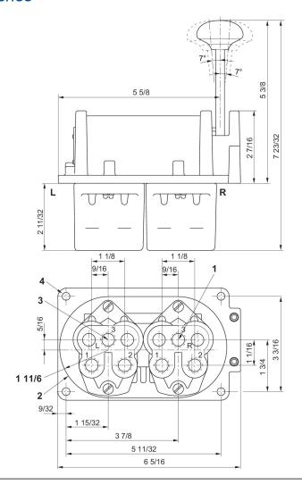
Triple 3-way valve - 3 position handle, detented
