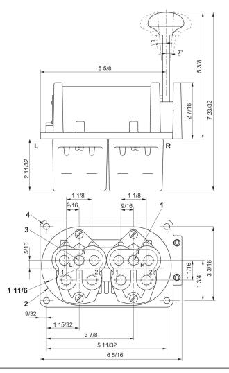
1) Air supply 2) Mounting hole 3) 1/4 - 18 NPTF 6 ports 4) 9/32 diameter (4) places
