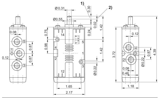
1) Stroke 2) Overstroke Dimensions of basic valve apply to all types of actuation.
