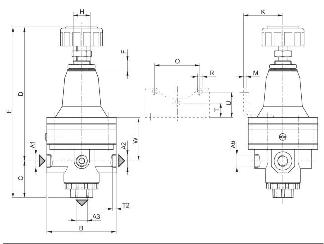
A1 = input A2 = output A3 = output A6 = output
