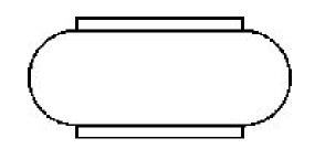
Max. permissible parallel movement between the covers: [[10] mm]
