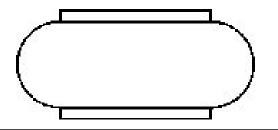
Max. permissible parallel movement between the covers: [[10] mm]
