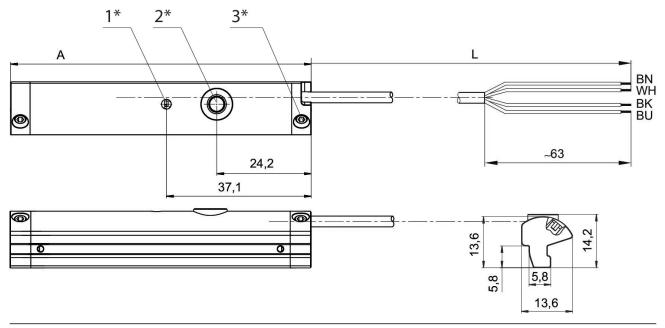
1\* = LED 2\* = teach button 3\* = threaded pin M3x11 L = cable length (2) WH=white A = sensor length
