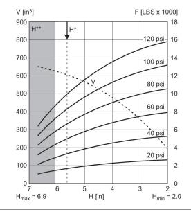
V = volume H = height H<sup>\*</sup> = recommended operating height for vibration isolation H<sup>\*\*</sup> = use permitted only upon approval by AVENTICS
