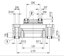
1) centering sleeve, included in the scope of delivery 2) centering sleeve
