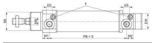
S=stroke 1) Slot in throttle screw 1 mm
