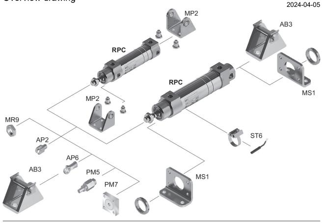
NOTE: This overview drawing is only for orientation to indicate where the various accessory parts can be fastened to the cylinder. The illustration has been simplified for this purpose. It is thus not possible to derive the dimensions from this overview.
