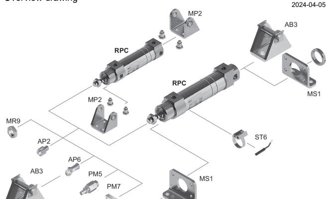
NOTE: This overview drawing is only for orientation to indicate where the various accessory parts can be fastened to the cylinder. The illustration has been simplified for this purpose. It is thus not possible to derive the dimensions from this overview.
