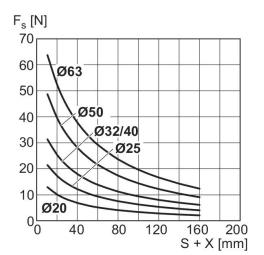
${\sf X}$  = distance between force application point and cylinder cover  ${\sf FS}$  = lateral force
