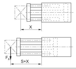
X = distance between force application point and cylinder cover FS = lateral force S = stroke
