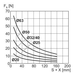
X = distance between force application point and cylinder cover FS = lateral force
