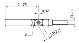
1\* = switching point 2\* = locking screw 3\* = LED window, transparent
