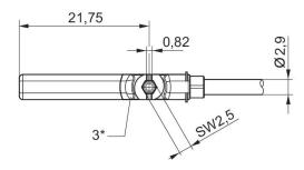
$1^*$  = switching point  $2^*$  = locking screw  $3^*$  = LED window, transparent L = cable length X = PNP: 11,6 mm, reed: 8,3 mm
